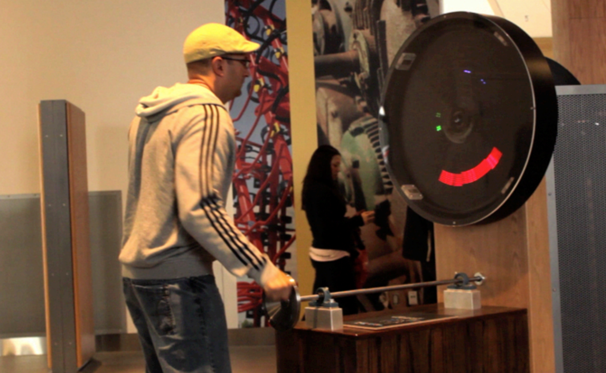
Generator - a flywheel generator that translate visitors' cranking action into electricity to power a LED persistence-of-vision display
